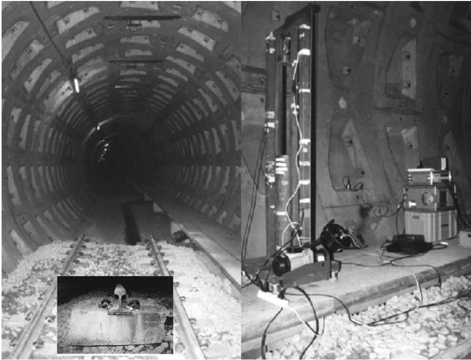
Fig. 11. Measurement set-up at pre-metro tunnel Herentalsebaan (Woodstraat crossing).
